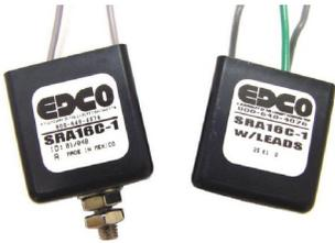
The **SRA16C-1** is a three terminal device, two of which are connected across the signal inputs of the detector for differential mode protection, and the third is grounded to protect against common mode damage.
